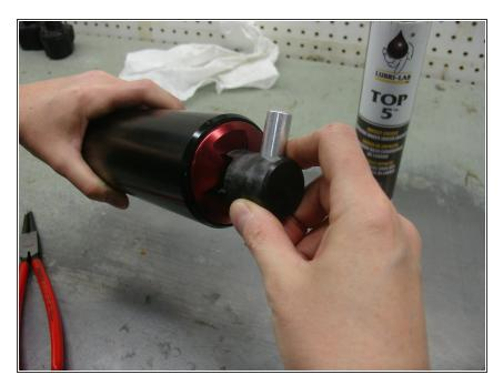
• Using the appropriate tool, unscrew to protector cap.
