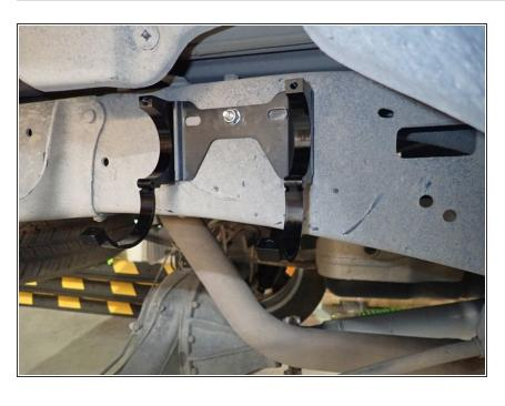
Install reservoir bracket with first supplied bolt in the hole already in frame at the right side of shock (right side shown)
