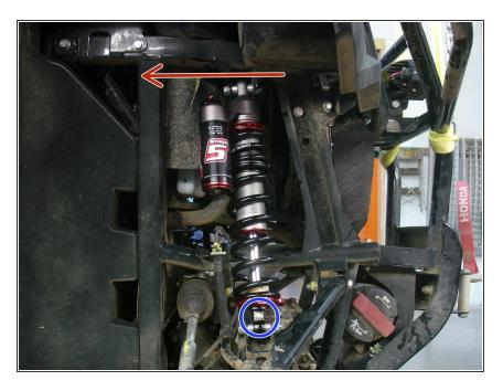
Install both new Elka front shocks with the piggyback reservoir at the top and oriented towards the rear
