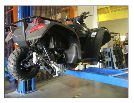
Lift the vehicle using a jack or stand so that the wheels are off the ground. Refer to your vehicle's owner manual for specific instructions on how to remove the stock shocks. Keep all the original hardware to re-use when installing your new Elka shocks.
