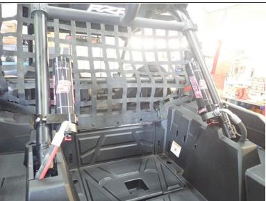
• Attach the reservoir to the rear of the roll cage as shown using the provided mounting bracket.
