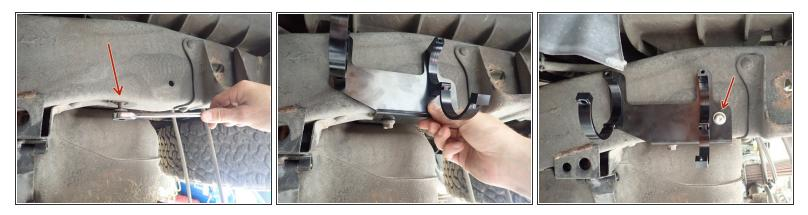
On the left side, use lower existing bolt to fix bracket, and use provided nylon-lock bolt in the existing hole to secure it.
