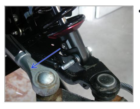
On Stage 2, Stage 4 and Stage 5 models, the lower shock eyelets should be installed with the rebound adjuster oriented towards the rear of the vehicle as shown by the blue Arrow on the photo (right side shown). If needed, you can turn the lower eyelet to orient properly.
