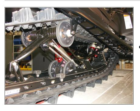
Install the Elka center shock with piggyback reservoir at the top and pointing towards the right side of
