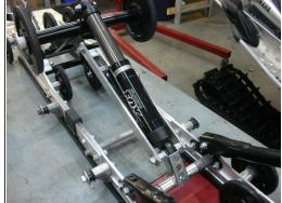
• Remove the 4 bolts of the rear skid, this step will give you a better access to the rear shock.
