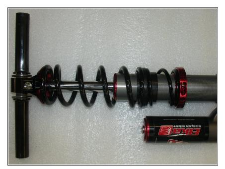
Install the sleeve through the bottom eye with the plastic spacer on both side of the eyelet.
