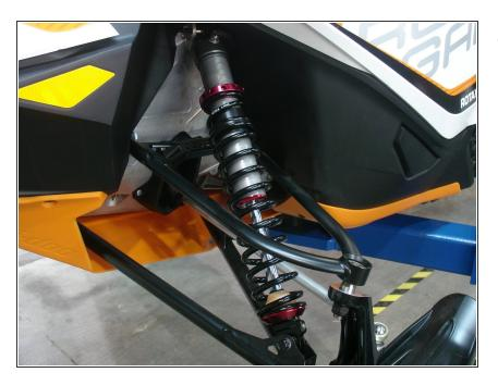
For Stage 2 front shocks, install with the Schraeder nitrogen valve oriented towards the side of the snowmobile as shown.
