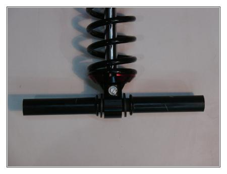
Install the sleeve through the bottom eye with the plastic spacer on both side of the eyelet.
