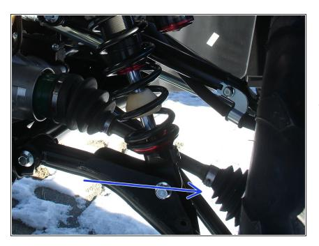
On Stage 2, Stage 4 and Stage 5 models, the lower shock eyelets should be installed with the rebound adjuster oriented towards the outside of the vehicle as shown by the blue Arrow on the photo (left side shown). If needed, you can turn the lower eyelet to orient properly.
