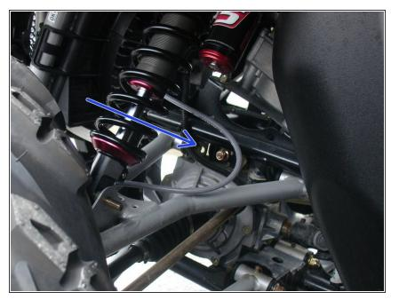
On Stage 2, Stage 4 and Stage 5 models, the lower shock eyelets should be installed with the rebound adjuster oriented towards the rear of the vehicle as shown by the blue Arrow on the photo ( left side shown ). If needed, you can turn the lower eyelet to orient properly.
