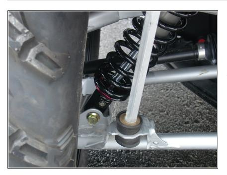
On Stage 2, Stage 4, and Stage 5 models the rebound adjuster located on lower eyelet of the shocks should be oriented towards the rear of the vehicle, as shown. (Left side shown ). If needed, you can turn the lower eyelet to orient properly.
