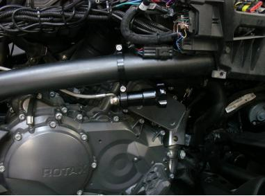
For hydraulic preload adjuster with a Stage 2 shock, fix bracket directly on frame as shown and torque the 2 bolts at 10 ft/pnds
