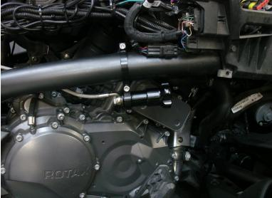
• For hydralic preload with a Stage 2 shock, fix the adjuster directly to the frame with supplied bracket as shown. Torque the 2 bolts at 10 ft/pnds.
