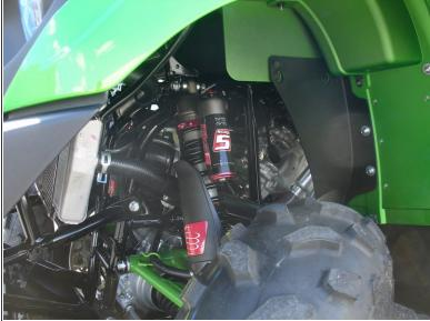
• Install the front new Elka shocks with the reservoir (on Stage 3-4-5) or Schraeder nitrogen valve (on Stage 1-2) at the top of vehicle. (left side shown).
