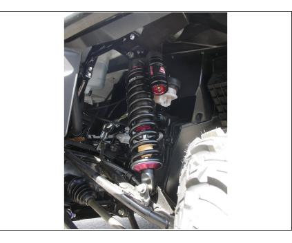
Install the front new Elka shocks with the reservoir (on Stage 3-4-5) or Schraeder nitrogen valve (on Stage 1-2) at the top of vehicle. ( left side shown).
